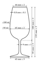
Fig. 3: Dimensions of ISO tasting glass
