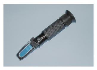
A portable refractometer
